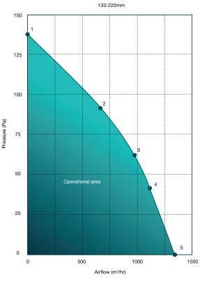
Tested in accordance with ISO 5801. Installation method - type A.
